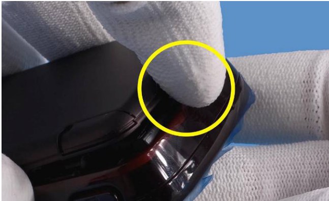
1. Press to release the BATTERY COVER .
