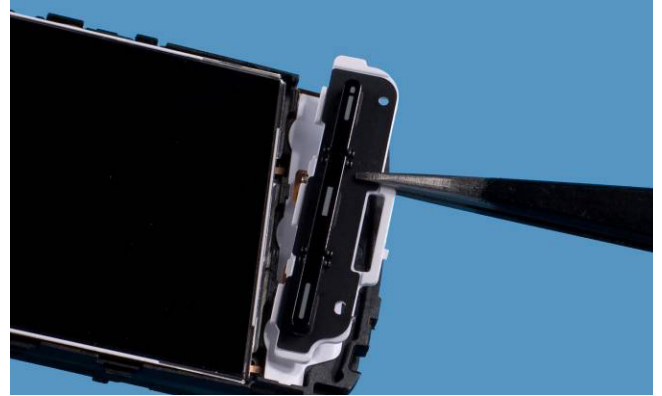
14. Use tweezers to remove KEYMAT .
