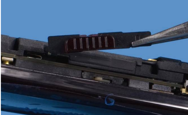
7. Use tweezers to remove SLIDE KEY .
