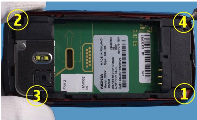
3. Unscrew the four TORX5+ screws.
